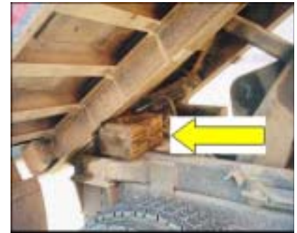
Figure 1 shows a wooden block makeshift body prop. Make-shift devices are not designed to safely support the elevated dump body.
